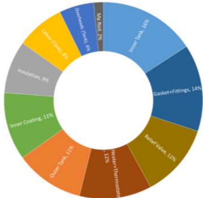
Figure 5.6 Breakdown of Storage Tanks Manufacturing Cost
