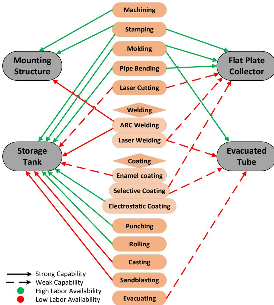
Figure 5.3 Linkages between components and manufacturing processes
