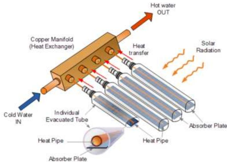
Figure 3.2 Evacuated tube collector typical breakdown components<sup>2</sup>
