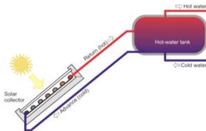
Figure 4.1 Functional diagram of a Thermosiphon system<sup>3</sup>
