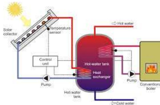
Figure 4.2 Functional diagram of a forced circulation system<sup>4</sup>
