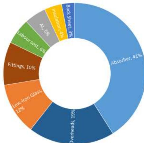
Figure 5.5 Breakdown of Flat Plate Collector Manufacturing Cost
